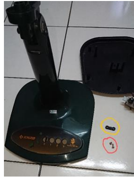
Figure 3: Elimination of wire holder screws and the wire holder is suggested to merge within the table fan's main body
