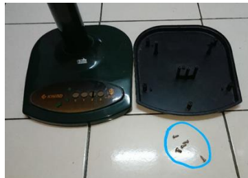
Figure 4: Reducing screws number from five to four
