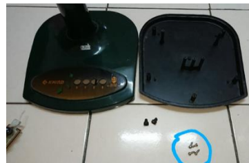
Figure 6: Reducing screws number from four to two as the supporters to support the snap-fit secure fitting
