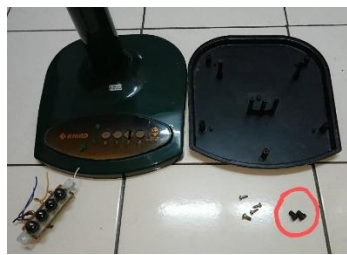
Figure 5: Elimination of rubber feet
