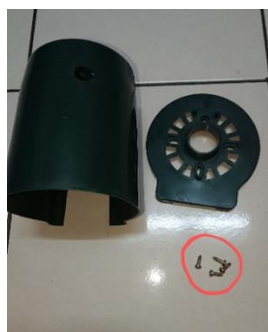
Figure 2: Elimination of motor housing screws
