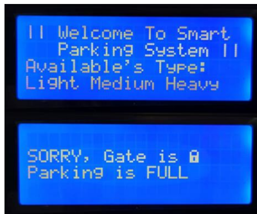
Figure 7: The main display of the system during available and fully occupied
