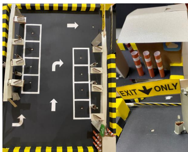
Figure 5: LDR sensor module mounted at parking slot, weather station and gate
