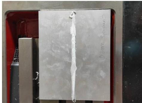
**Figure 6: Friction Stir Welded Plate**
