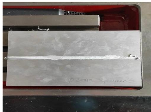
Figure 11: Specimen C with Tool Pin Diameter of 3 mm
