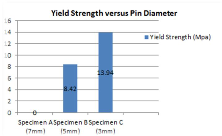
**Figure 14: Graph of Yield Strength vs Pin Diameter**
