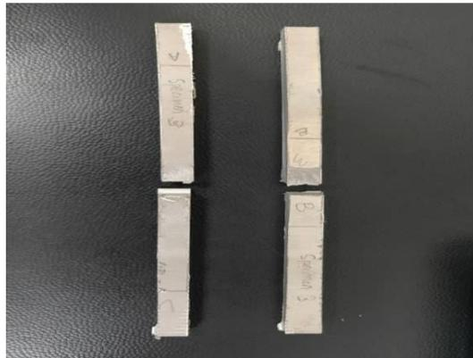
**Figure 8: Tensile Tested Specimen**
