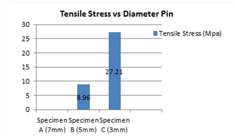
Figure 12: Graph of Tensile Stress vs Diameter Pin
