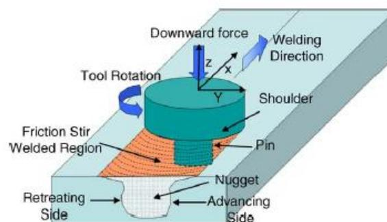
**Figure 4: Working Principle of FSW**
