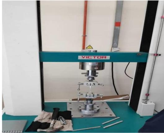
**Figure 7: Victor Universal Testing Machine**
