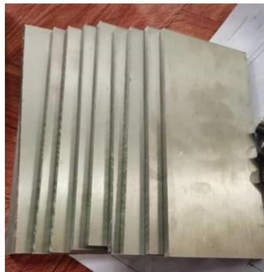
Figure 1: Aluminium A1100 (200 mm x 75 mm x 6 mm)
