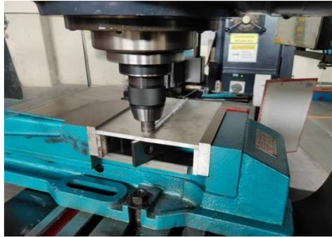
**Figure 5: Welding by FSW**
