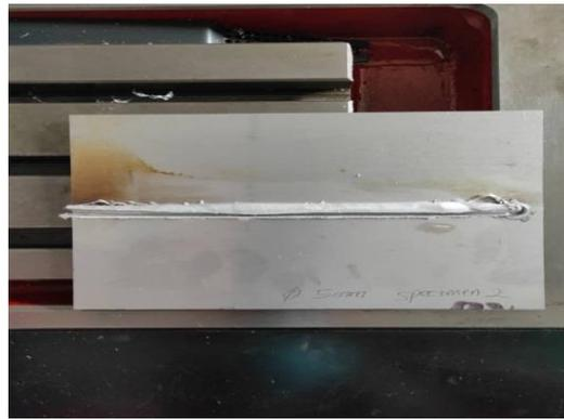
Figure 10: Specimen B with Pin Tool Diameter of 5 mm
