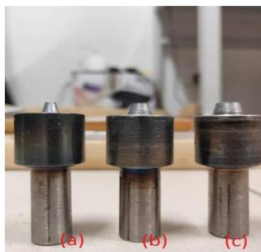
Figure 2: Conical Pin with different Diameter (a) 3 mm, (b) 5 mm, (c) 7 mm
