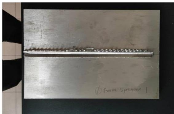
**Figure 9: Specimen A with Pin Tool Diameter of 7 mm**
