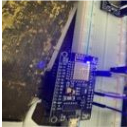
Figure 9: NodeMCU ESP8266 built in LED is blinking
