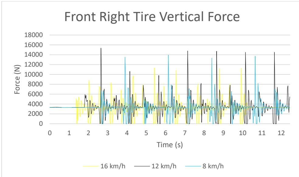
**Figure 12: Front Right Tire Vertical Force**
