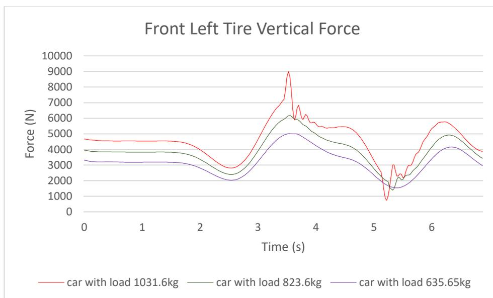
**Figure 18: Front Left Tire Vertical Force**
