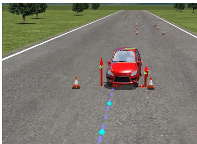
**Figure 7: Animation on Double Lane Change Test at 110 km/h**
