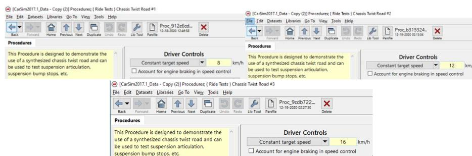
**Figure 3: Vehicle Speed Setup in Procedure Section: Chassis Twist Road in CarSim®**
