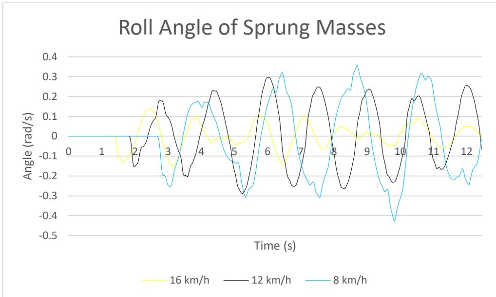
**Figure 10: Roll Angle of Sprung Mass**
