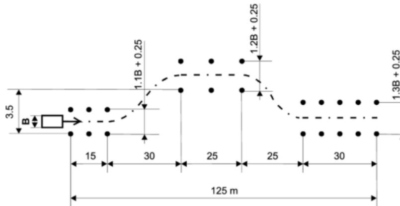
**Figure 5: The Track of the Double Lane-Change Maneuver in Accordance with Standard No. ISO 3888:1975 [9]**
