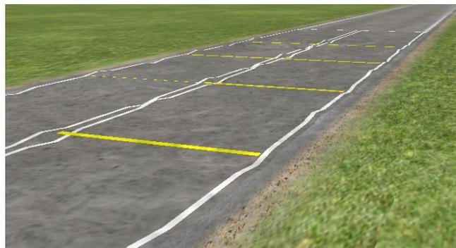
**Figure 2: Chassis Twisted Road Profile**
