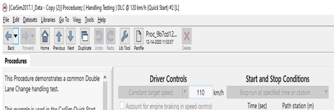
**Figure 6: The Vehicle Speed Setup for Double Lane Change Procedure in CarSim® Software**
