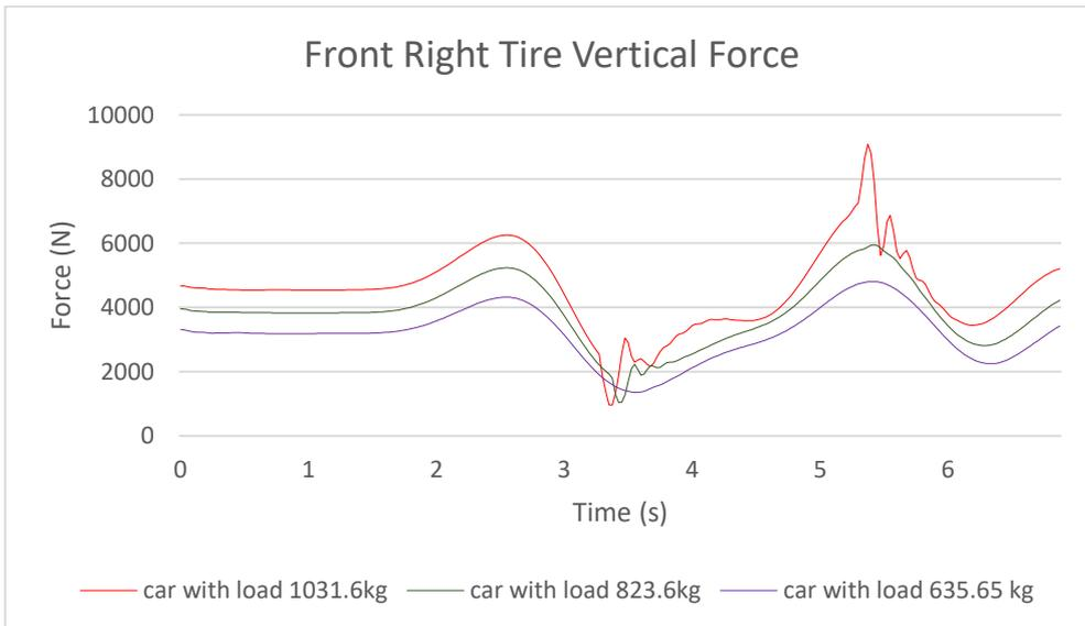
**Figure 17: Front Right Tire Vertical Force**
