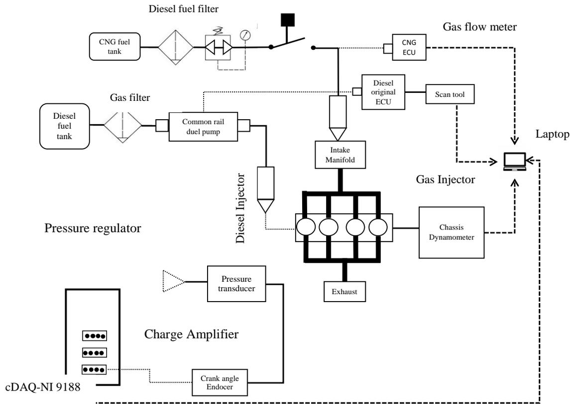
**Figure 2: Schematic Diagram for experiment Setup**
