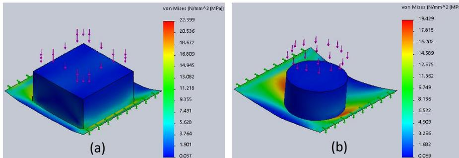
**Figure 9: Stress on plastic film after acted on (a) 5.0 kg (square base) and (b) 5.0 kg of load (cylinder base)**
