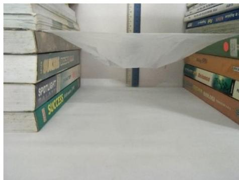
**Figure 7: The plastic film was deformed after the 5.0 kg of load unloaded**
