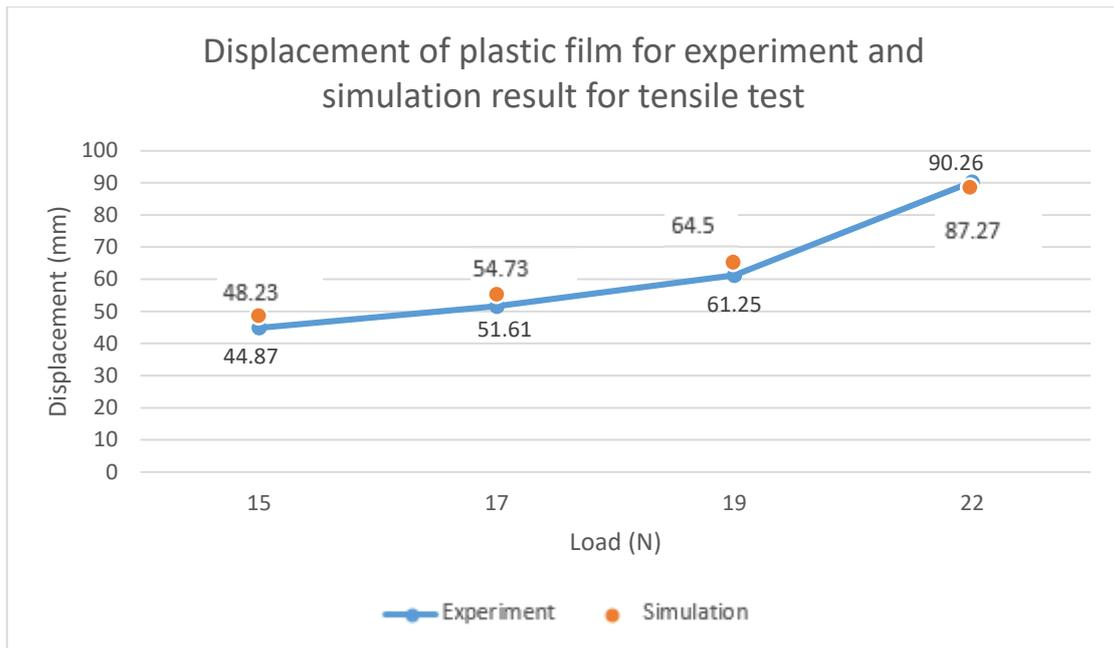
**Figure 5: Displacement of plastic film for experiment and simulation results for the tensile test**
