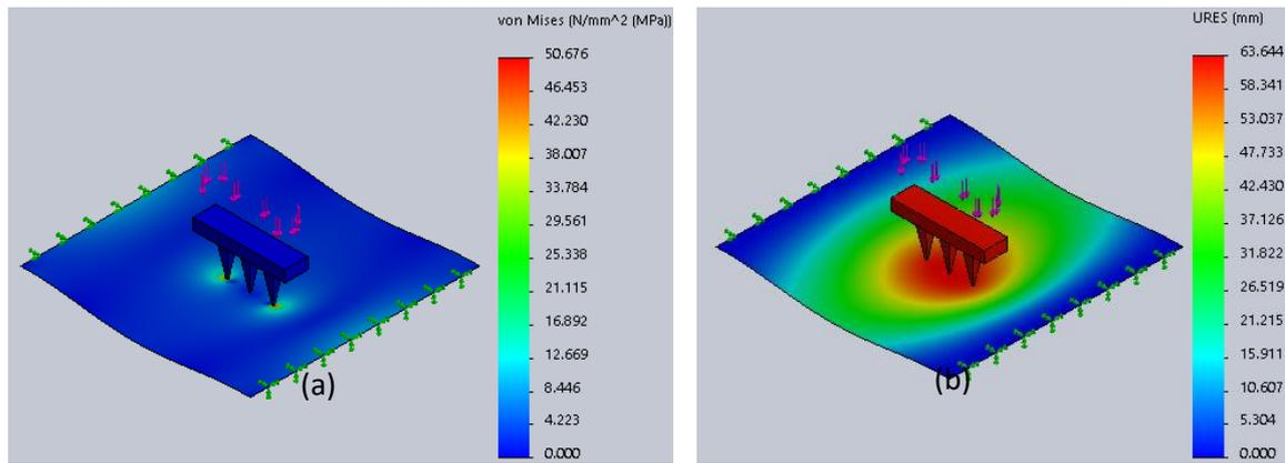
**Figure 11: (a) The plastic film towards point stresses (b) displacement of the plastic film after acted by sample G**
