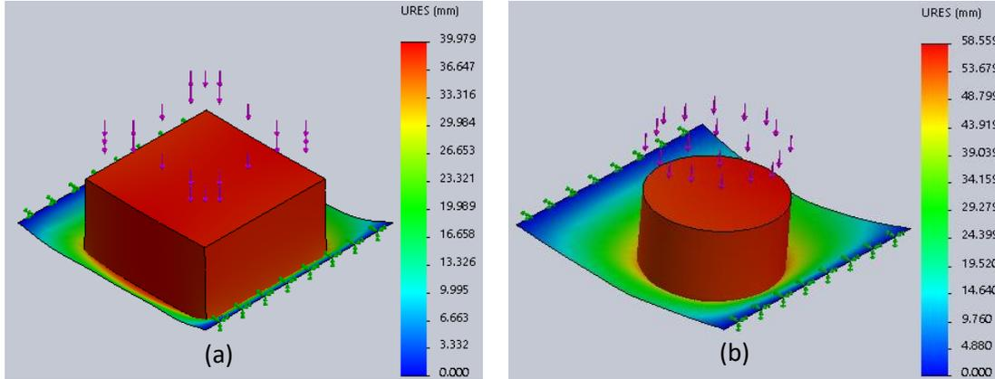
**Figure 8: Displacement of plastic film with (a) 5.0 kg (square base) and (b) 5.0 kg of load (cylinder base)**
