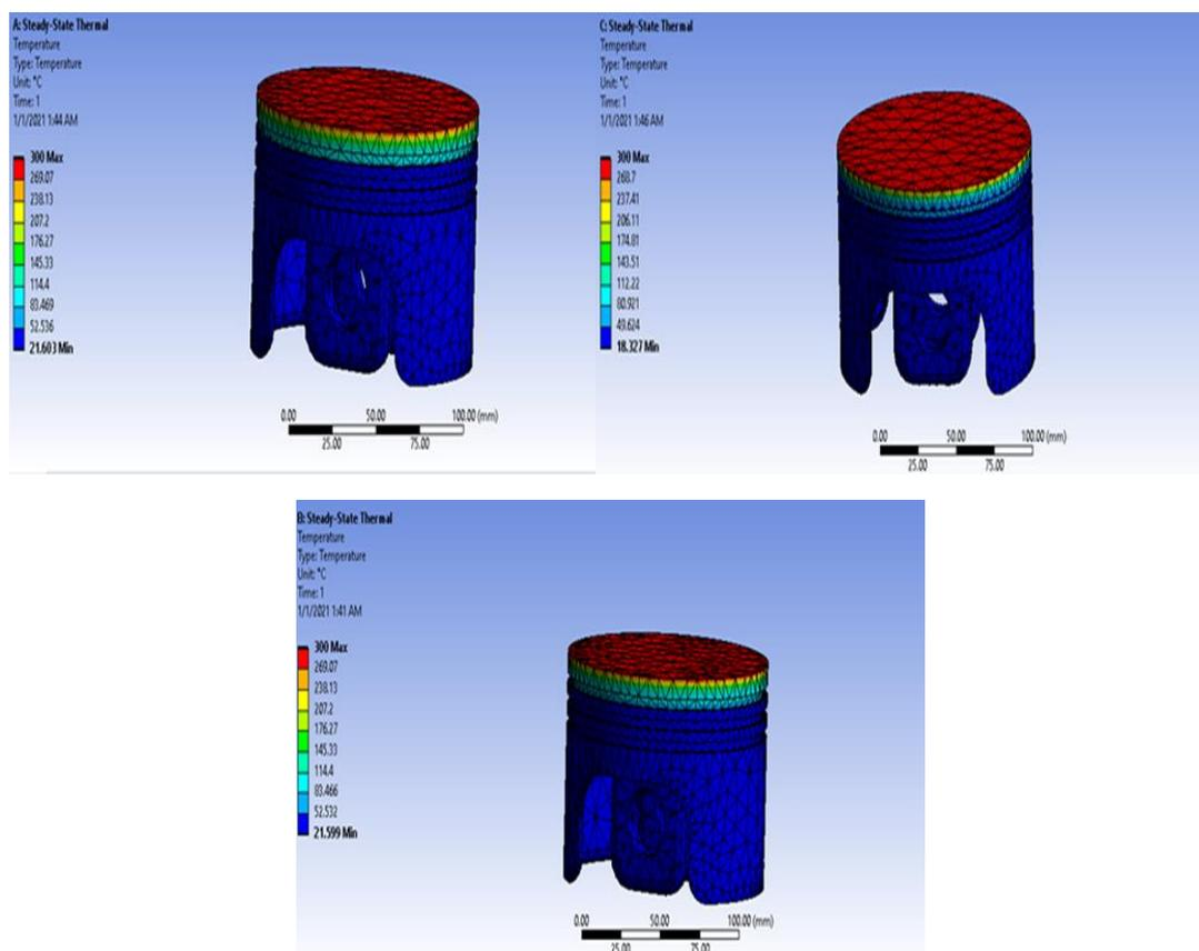
**Figure 5: Temperature Distribution of Al Alloy, Gray Cast Iron and Si-C in Steady State Thermal**
