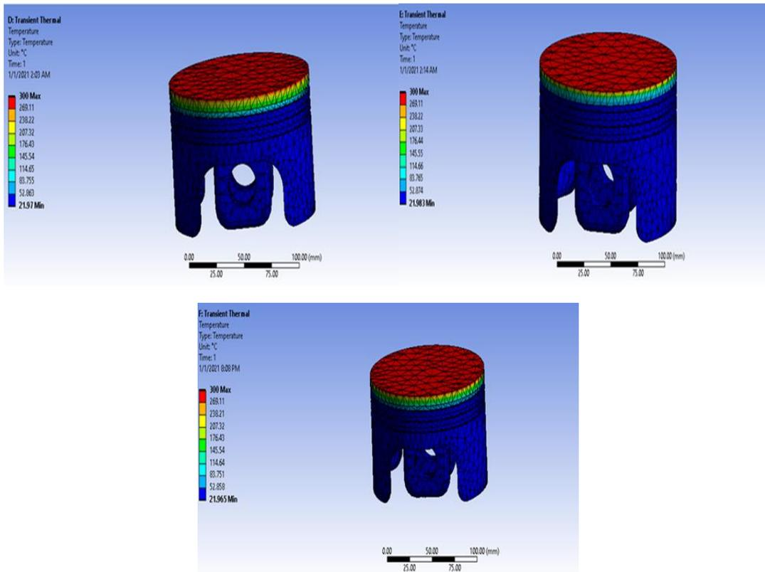
**Figure 6: Temperature Distribution of Al Alloy, Gray Cast Iron and Si-C in Transient Thermal**
