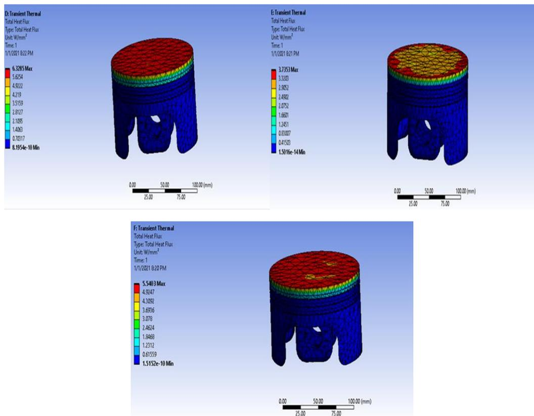
**Figure 7: Total Heat Flux of Al Alloy, Gray Cast Iron and Si-C**
