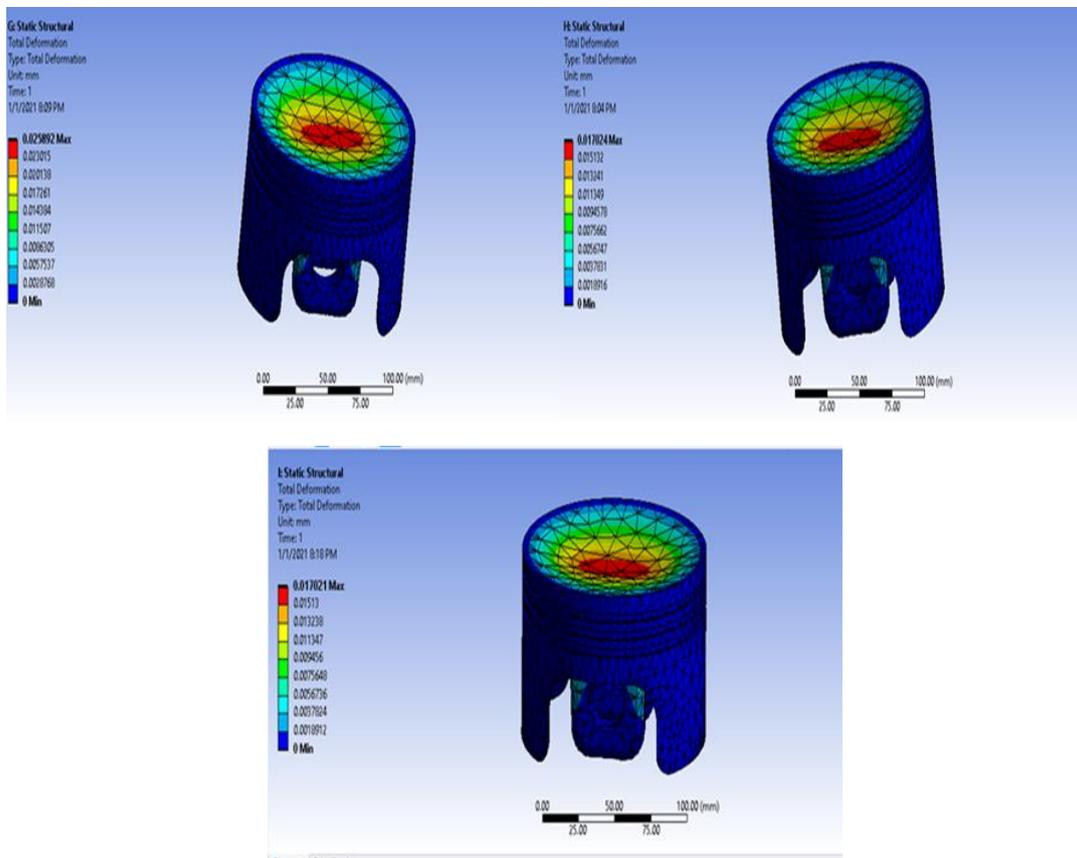
Figure 4: Total Deformation of Aluminium Alloy, Gray Cast Iron and Si-C (MMC)
