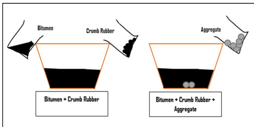
**Figure 3: Wet method process**
