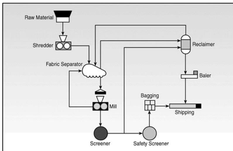
Figure 4: Crumb Rubber Process [4]
