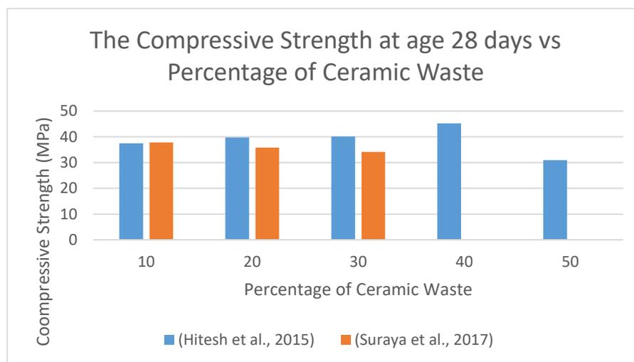
**Figure 5: Bar Chart of compressive Strength at 28 days**
