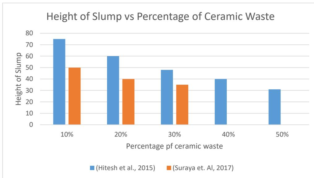
**Figure 3: Bar chart for slump test**
