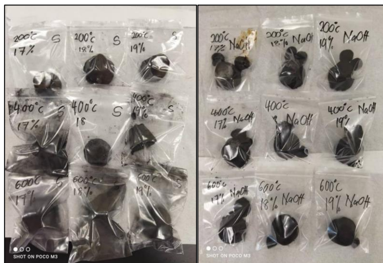
Figure 2: Palm kernel shell briquettes for starch binder on the left and palm kernel shell briquettes for NaOH binder on the right
