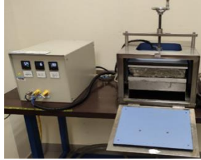
Figure 3: Guarded hot plate technique
