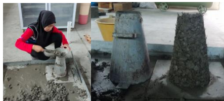
Figure 2: Slump testing process
