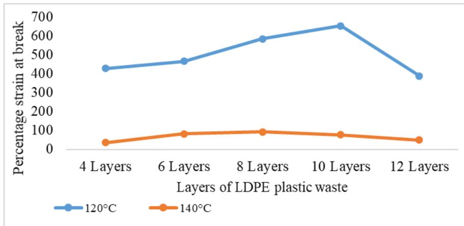
**Figure 4: Percentage strain at break of different layer of LDPE plastic bag waste**
