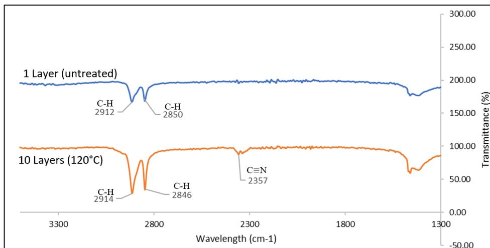
**Figure 7: Comparison of FTIR result of 1 layer and 10 layers of LDPE plastic bag waste**
