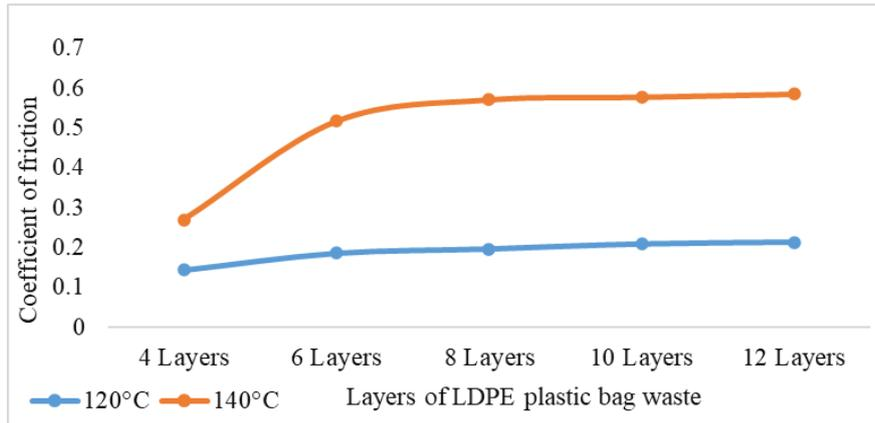
**Figure 6: Coefficient of friction by geotextile sample**
