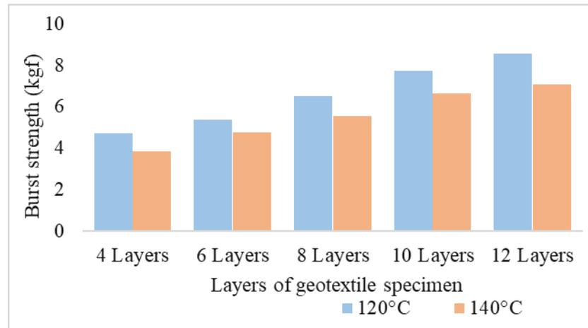
**Figure 5: Burst strength by geotextile sample layers**
