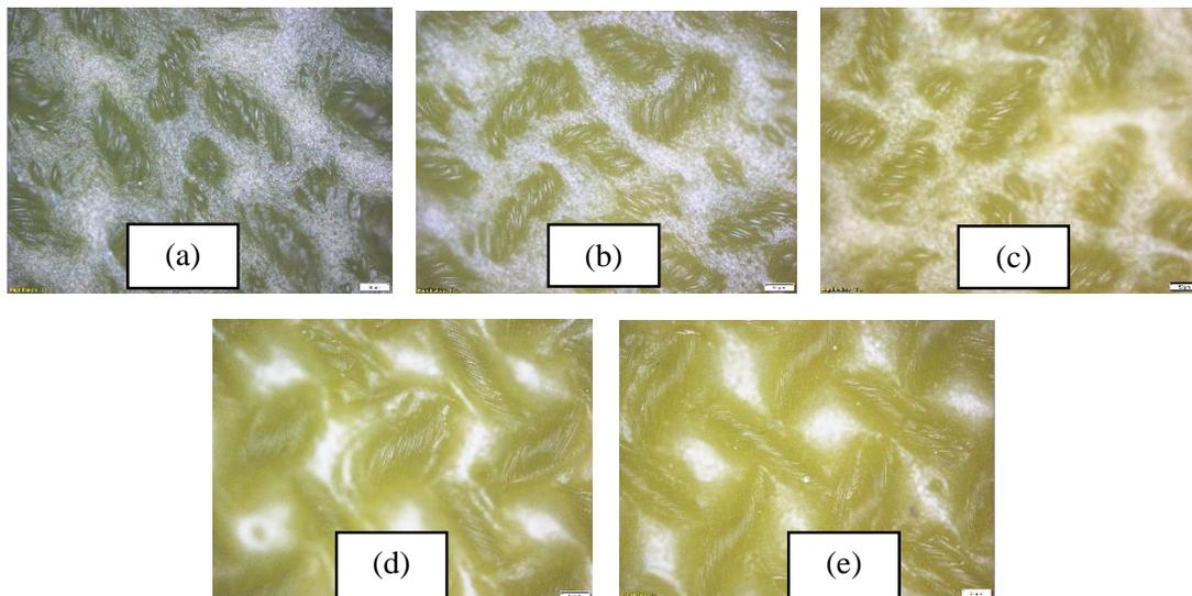
**Figure 10: Geotextile samples that undergoes 140°C heat transfer process; (a) 4 layers; (b) 6 layers; (c) 8 layers; (d) 10 layers; and (e) 12 layers**
