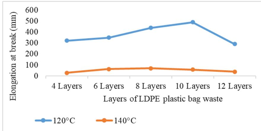
**Figure 3: Elongation at break, mm of different layer of LDPE plastic bag waste**
