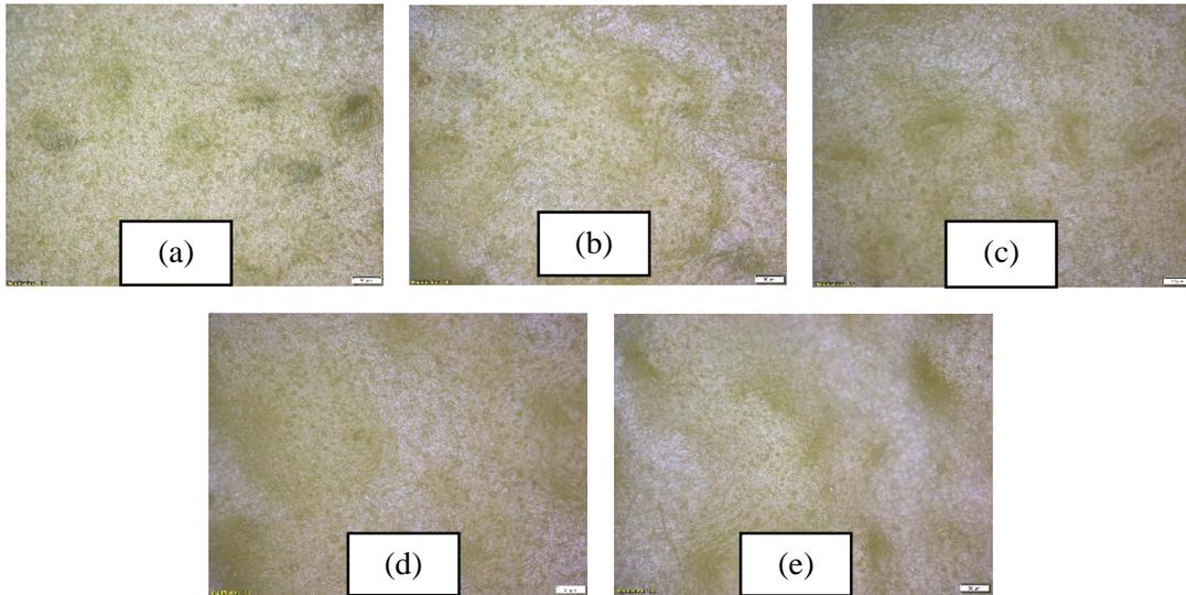
**Figure 9: Geotextile samples that undergoes 120°C heat transfer process; (a) 4 layers; (b) 6 layers; (c) 8 layers; (d) 10 layers; and (e) 12 layers**
