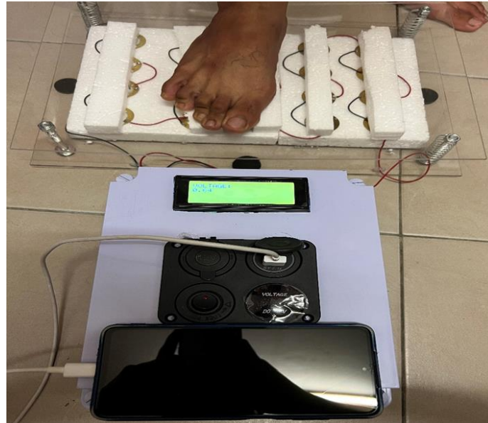
Figure 7: Analysis on the piezoelectric tiles
