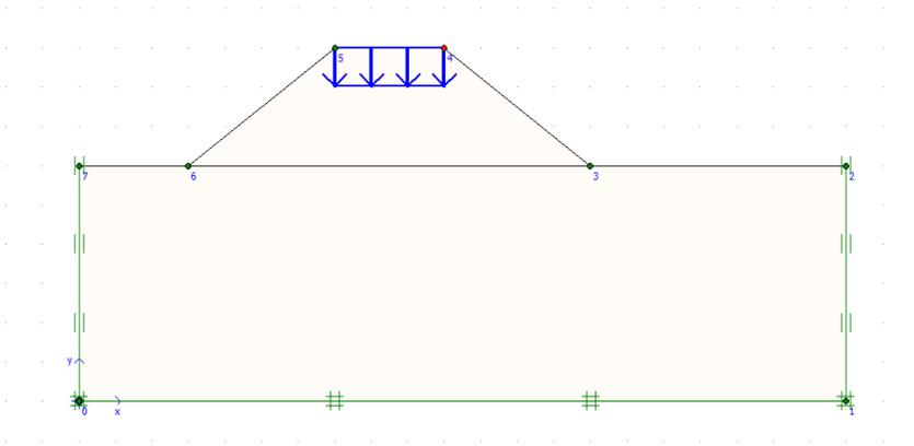
**Figure 3: Prescribe displacement at the top of the embankment**
