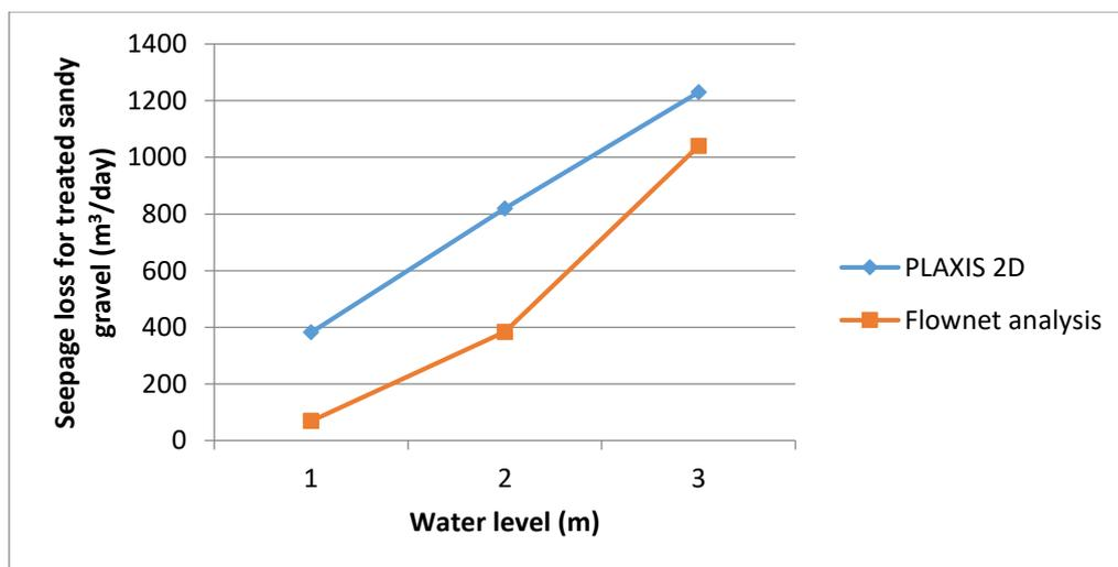
**Figure 8: Graph of water level vs. seepage loss for treated sandy gravel**
