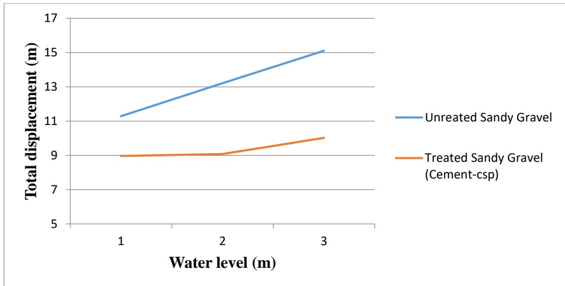
Figure 4: Graph of water level (m) vs total displacement (m)
