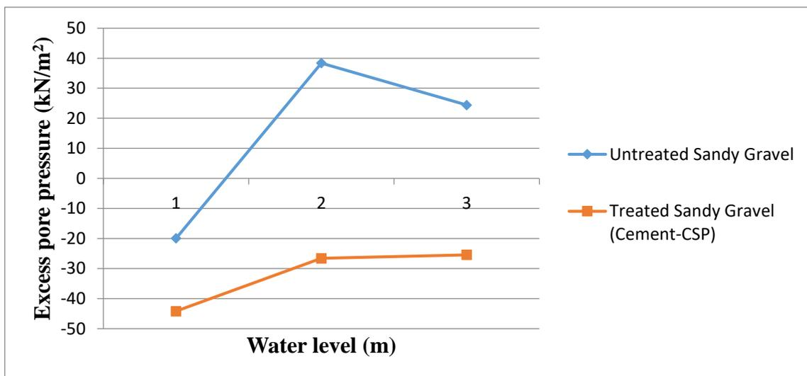
**Figure 6: Graph of water level (m) vs. Excess pore pressure (kN/m<sup>2</sup>)**
