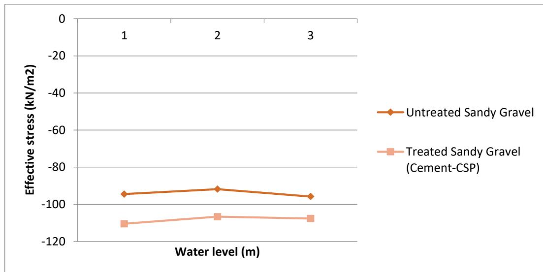
Figure 5: Graph of water level (m) vs. Effective stress (kN/m<sup>2</sup>)
