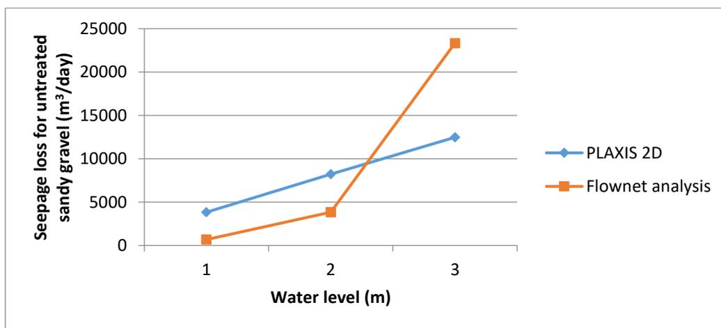
**Figure 7: Graph of water level vs. seepage loss for untreated sandy gravel**
