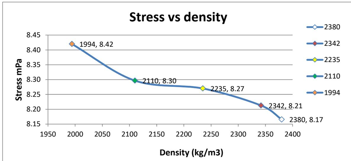
**Figure 10: The graph of Stress against Density for concrete beam model**
