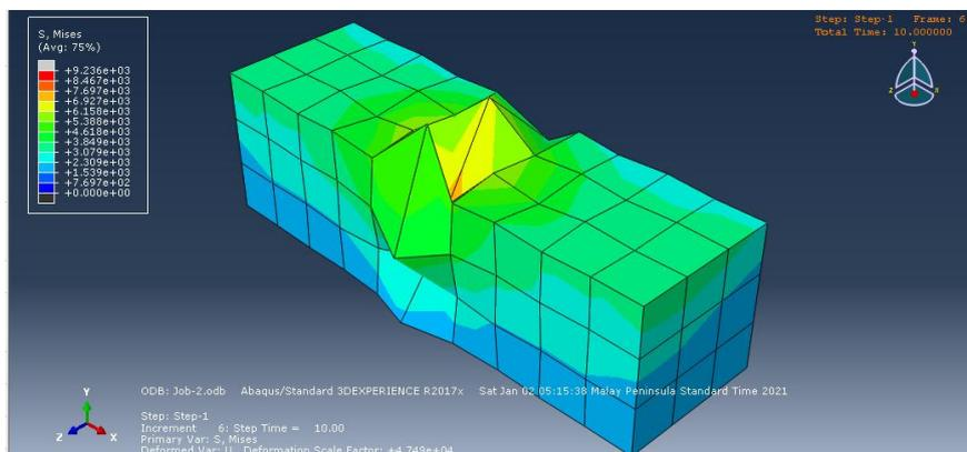
**Figure 8: The deformation pattern for concrete beam containing 20.00 % POFA and 30.00 % EPS**
