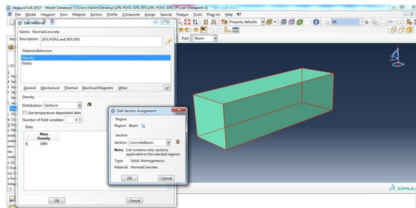
**Figure 2: Assign the material in model**
