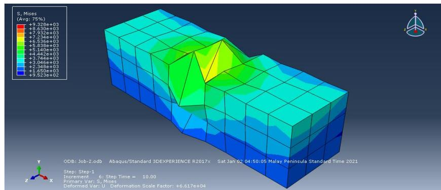
**Figure 7: The deformation pattern for concrete beam containing 20.00 % POFA and 0.00 % EPS**
