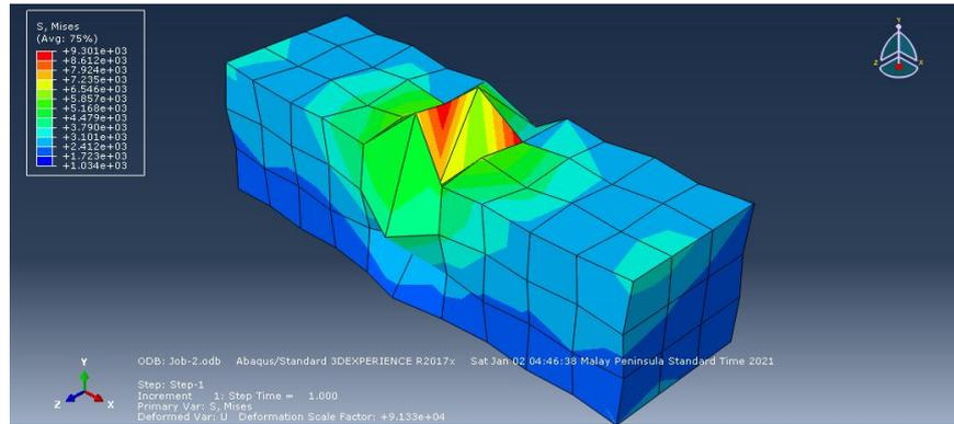
**Figure 6: The deformation pattern for normal concrete beam**
