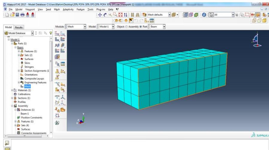
**Figure 3: Mesh the concrete beam model**
