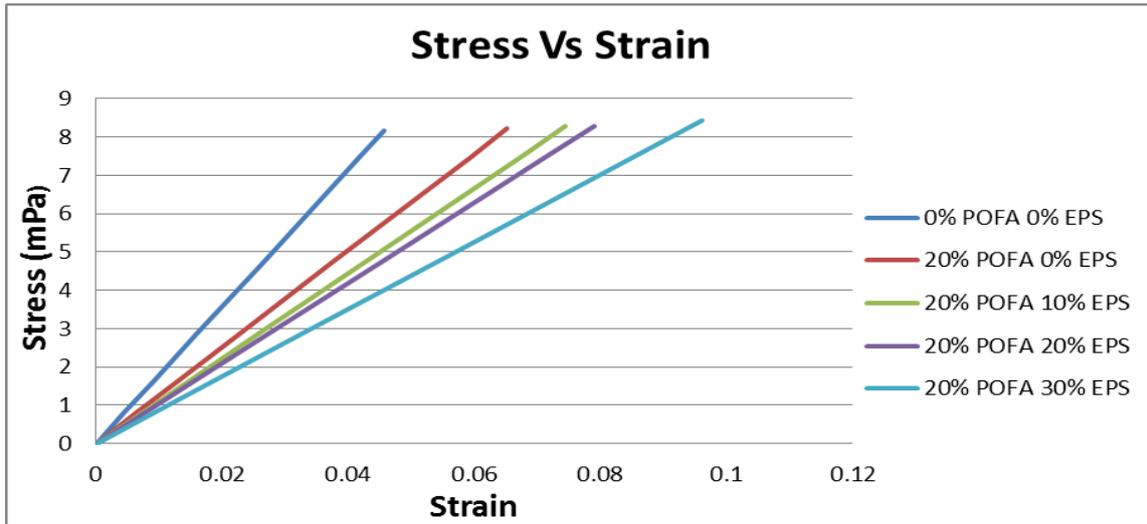
Figure 9: The graph of Stress vs Strain for concrete beam model
