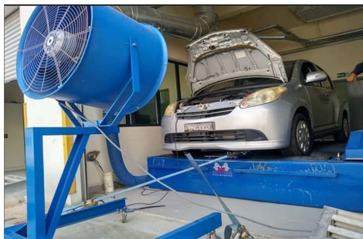
Figure 4: Test Vehicle Is Being Engage with The Belts on Dynamometer
