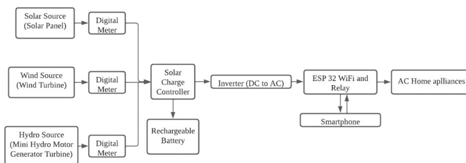
**Figure 1: Block Diagram**
