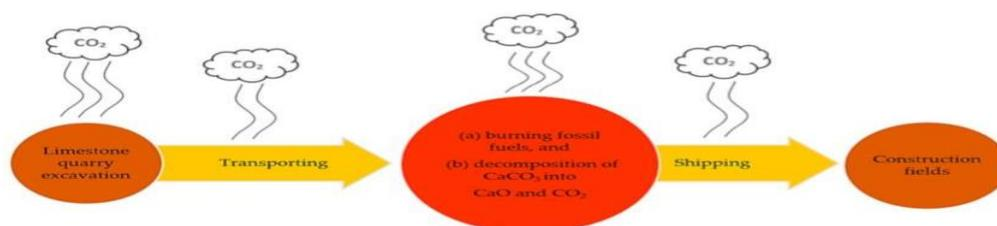
Figure 1: Shows main output and processes for OPC [5]
