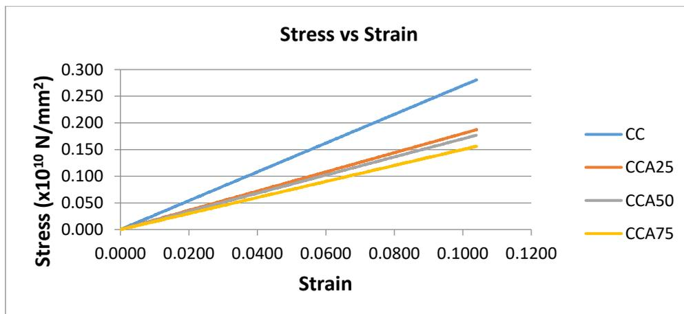
Figure 9: Graph of stress against strain for concrete cube model
