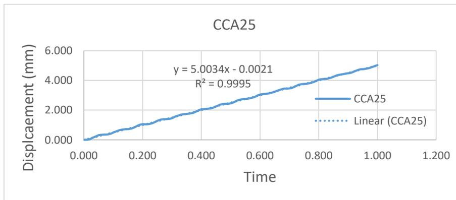
**Figure 11: Graph of displacement against time for CCA25 cube model**
