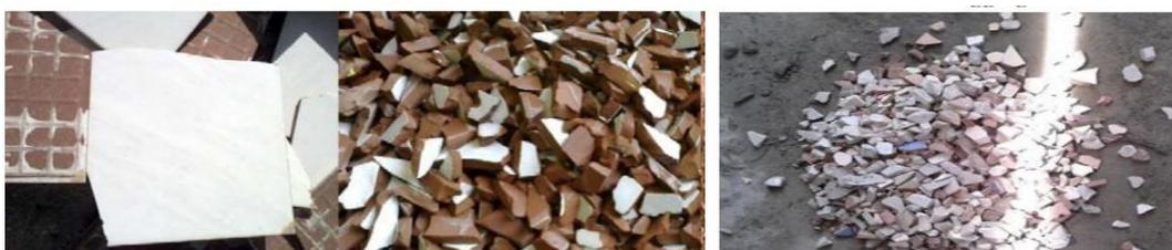
**Figure 3: Example of ceramic wastes [8]**
