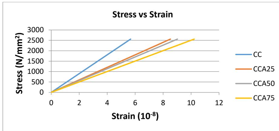
**Figure 15: Graph of stress against strain for concrete prism beam model**
