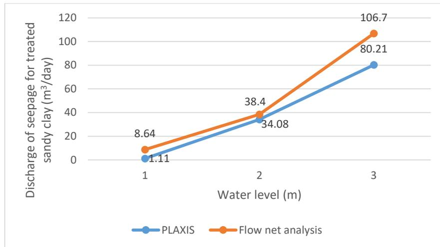
**Figure 10: Graph of water level vs discharge of seepage for treated sandy clay**
