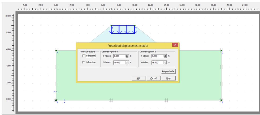
Figure 5: The prescribed displacements dialog box in the staged construction window
