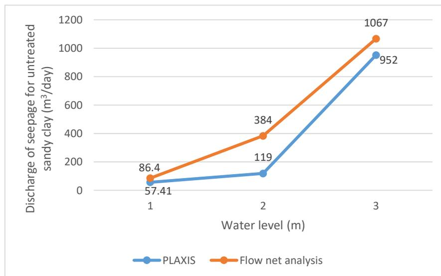
**Figure 9: Graph of water level vs discharge of seepage for untreated sandy clay**
