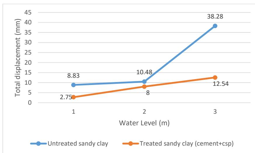
**Figure 6: Graph of water level vs total displacement**
