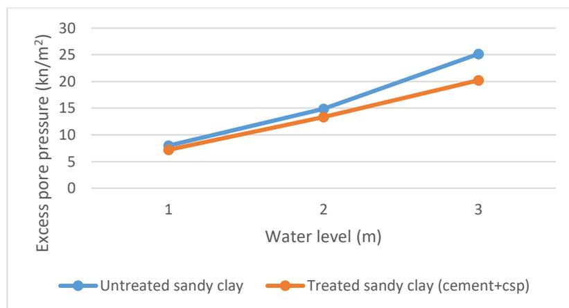
**Figure 8: Graph of water level vs excess pore pressure**
