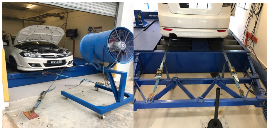
Figure 9: Front and Rear Vehicle Setup on Dynamometer
