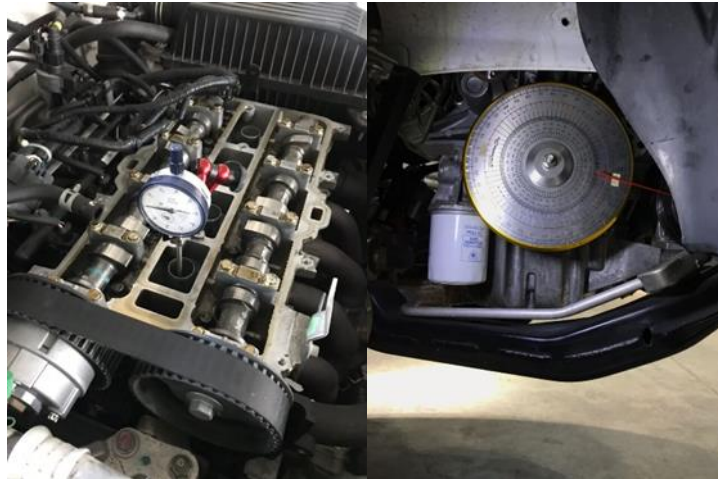
Figure 5: Dial gauge placed on piston surface and degree wheel attached on crank shaft pulley
