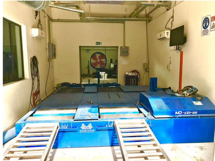
Figure 4: Mustang Chassis Dynamometer (MD-AWD-500)
