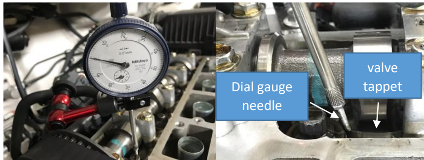
Figure 7: Dial gauge attached, and needle placed above inlet valve tappet
