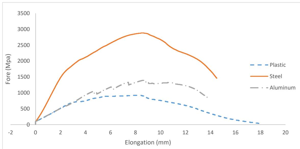
**Figure 8: Force-elongation curve for sandwich composite reinforcement**
