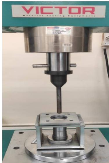
**Figure 5: Universal Tensile Machine**
