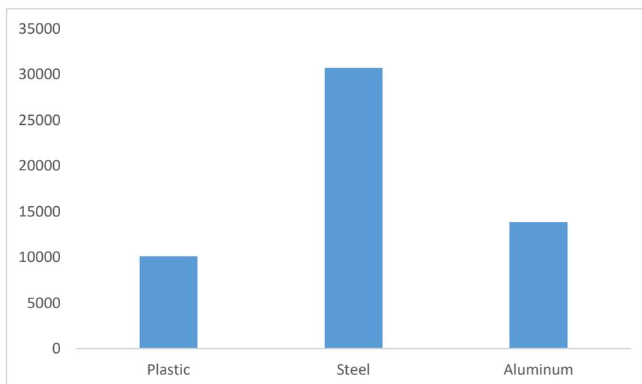
**Figure 10: Total energy absorption obtain from sandwich composite reinforcements**
