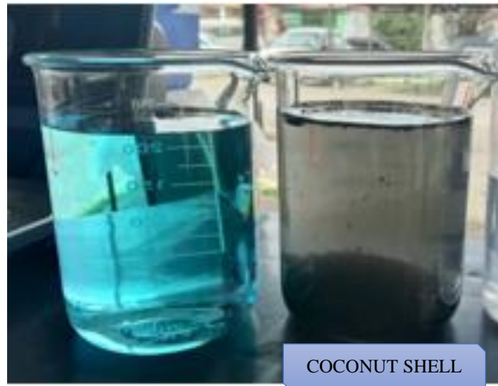
Figure 4: Decolored methylene blue after being adsorbed by coconut shell activated carbon
