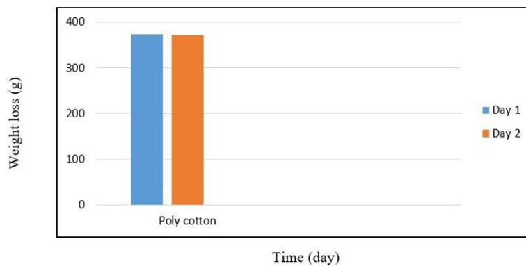
**Figure 1: Graph of weight loss (g) against time (day) for moisture vapor transmission**
