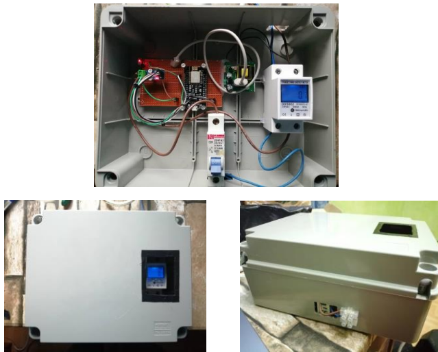
Figures 6: Prototype of IoT Based Power Monitoring Device (Distribution Box)
