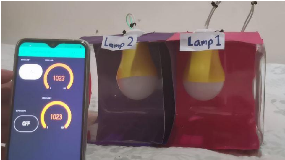
Figure 9: Status Lamp 1 on when Button Lamp 1 press but blub was light off
