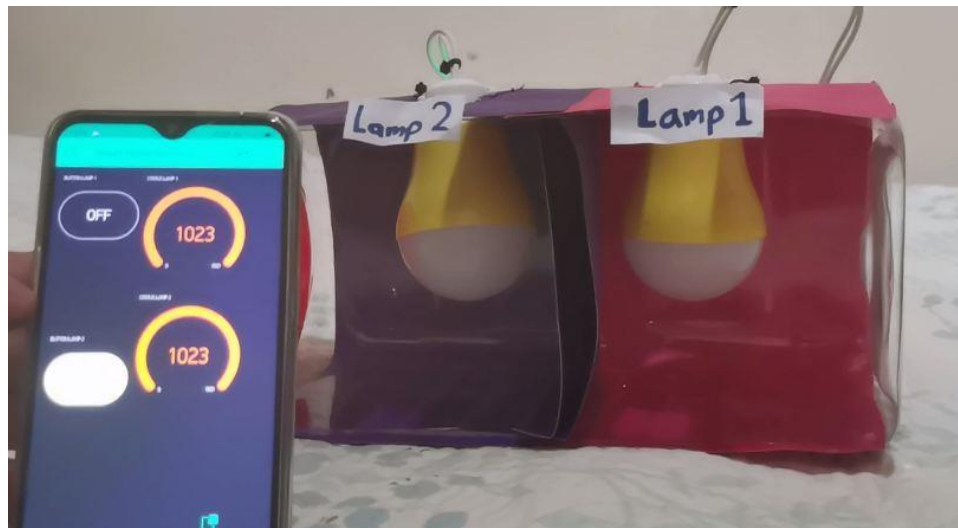
Figure 10: Status Lamp 2 on when Button Lamp 2 press but blub was light off
