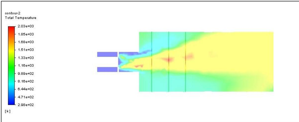
**Figure 3: Temperature contour for axial swirler.**
