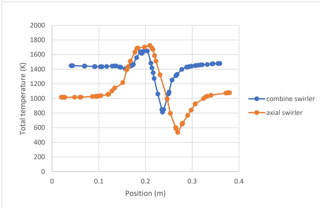
**Figure 4: comparison of total temperature for combine swirler and axial swirler at 0.065 m**
