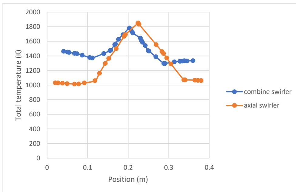
**Figure 6: Comparison of total temperature for combine swirler and axial swirler at 0.200 m**
