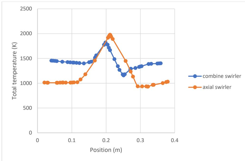
**Figure 5: comparison of total temperature for combine swirler and axial swirler at 0.130 m**
