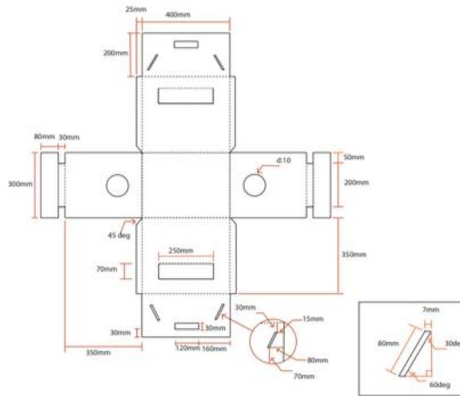
**Figure 11: Die cut drawing of PCTB**
