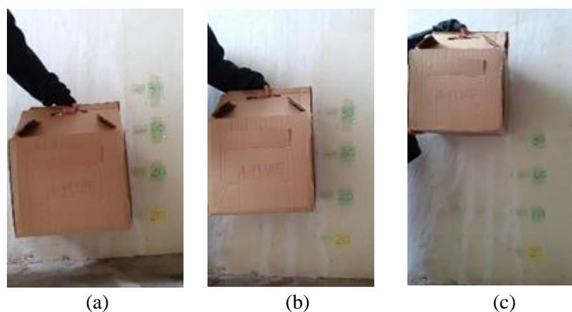
**Figure 5: Drop test set-up (a) 200 mm (b) 400 mm (c) 800 mm**
