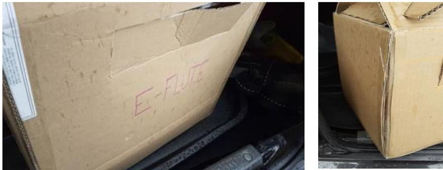
**Figure 15: Defects on E-Flute PCTB at 60 km/hours**
