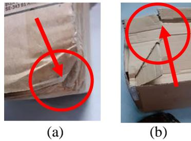
Figure 13: B-Flute and E-Flute drop and lift test defects (a) drop (b) lift-handle area
