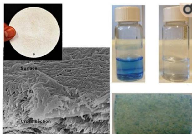
**Figure 4: the visual appearance of freeze-dried membranes and SEM images showing the CNCs on the surface and bulk of the membrane. The membranes adsorbed 98.0 % of Victoria blue 2B from water**
