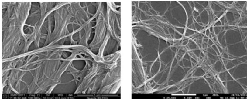
**Figure 3: SEM images of MFC (left) and NFC (right) [25]**
