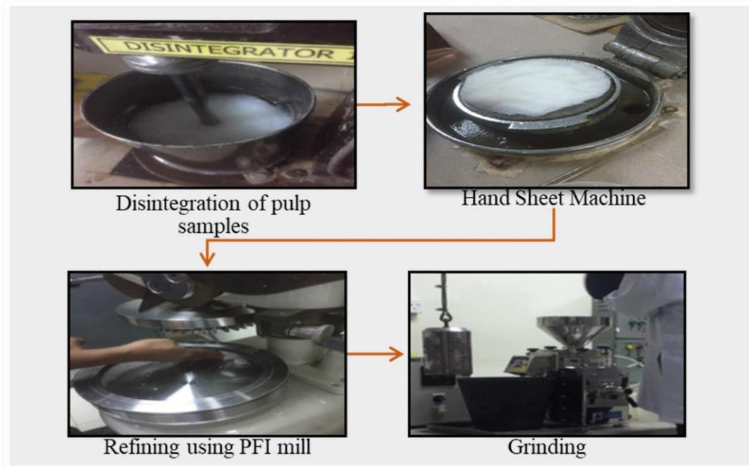
**Figure 1: The process of Nanofibrils cellulose (NFCs) preparation**
