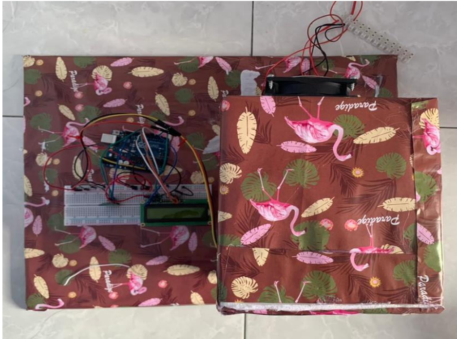
Figure 8: The top view of the prototype of the thermoelectric mini-portable fridge with a wireless temperature monitoring
