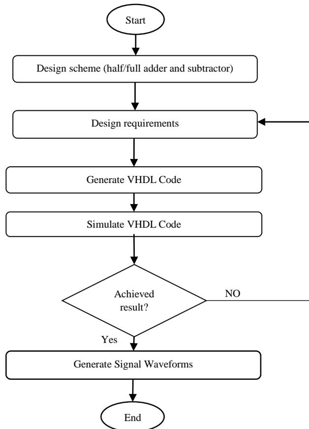
Figure 3: Flow chart of reversible binary half and full adder and subtractor
