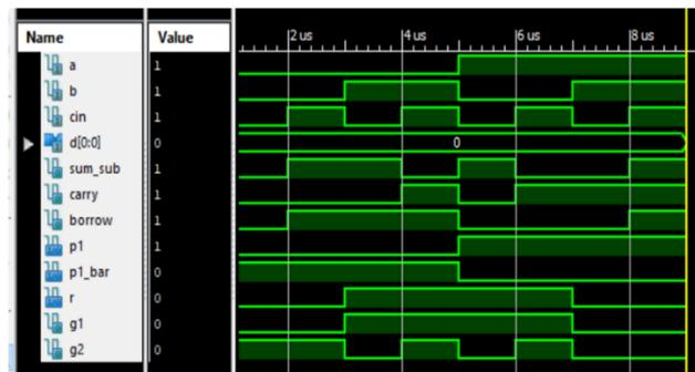
Figure 7: Waveform of reversible binary full adder/subtractor
