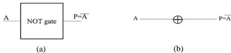
**Figure 1: Reversible NOT gate (a) symbol and (b) the quantum representation**
