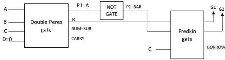
Figure 5: Block diagram of reversible full adder/subtractor
