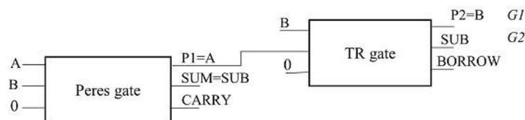
Figure 4: Block diagram of reversible half adder/subtractor
