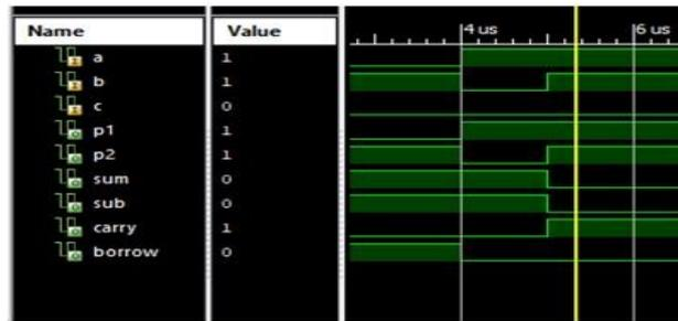
Figure 6: Waveform of reversible binary half adder/subtractor
