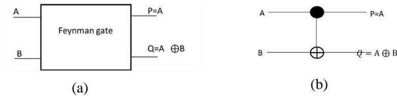
**Figure 2: Feynman gate (a) symbol and (b) the quantum representation**
