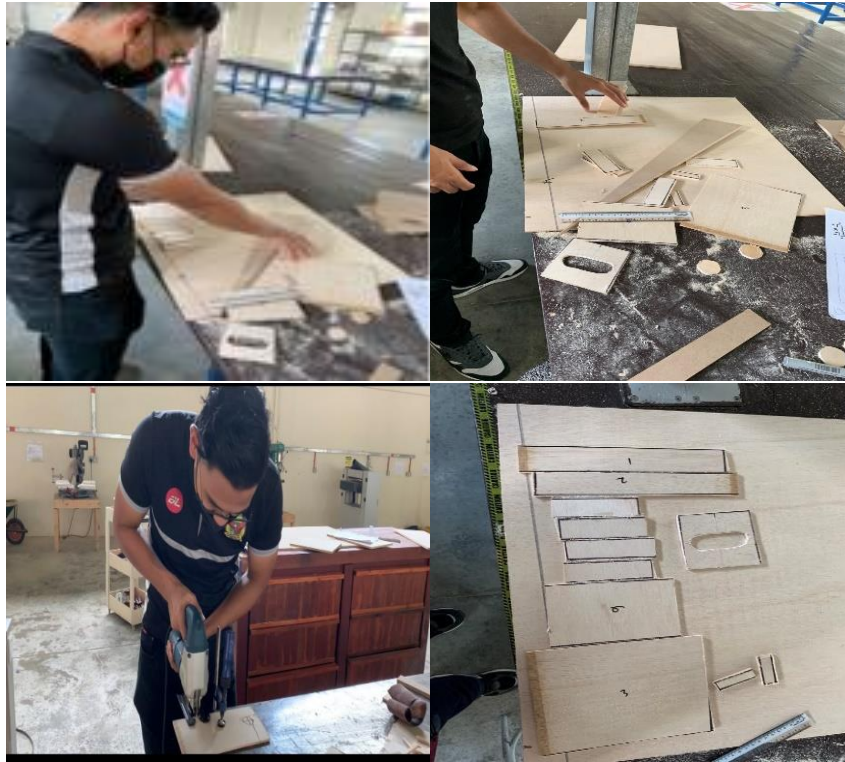
Figure 4: (a) Dimensional measurement; (b) Marking process; (c) Hand-held jig saw cutting; (d) Cutting into desired shape
