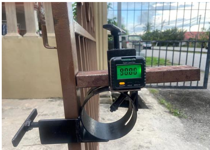
Fig. 2 Portable Electronic Angle List Finder used on iron grilles
