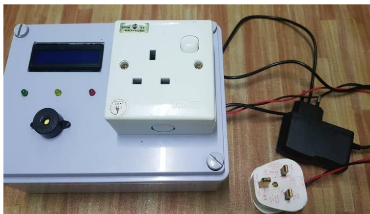
Figure 4: The current and power reading detector
