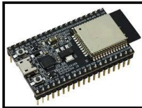
**Figure 3: ESP32 Micro Board**
