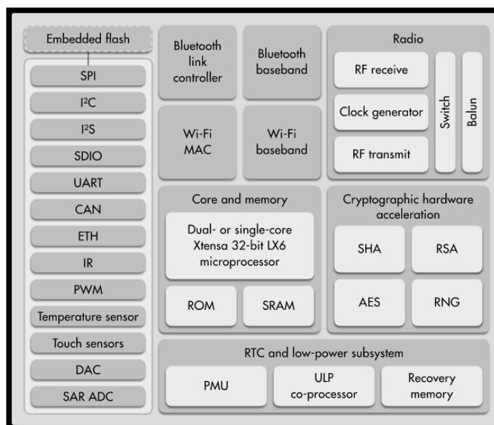
**Figure 4: Functional block diagram for ESP32 microboard**
