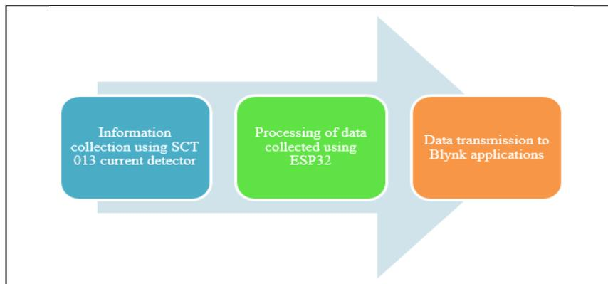
**Figure 1: Block diagram of energy consumption monitoring system using IoT**
