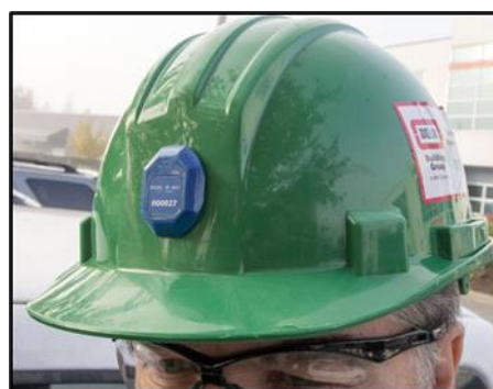
Figure 1: Helmet with GuardRFID AT-4 active tag (RFID Journal, 2014)
