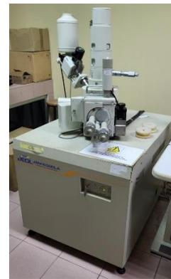
**Figure 8 JOEL JSM-6380LA Scanning Electron Microscope**
