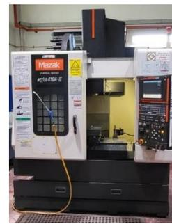
**Figure 4 YAMAZAKI MAZAK VCN-410-II CNC Milling Machine**
