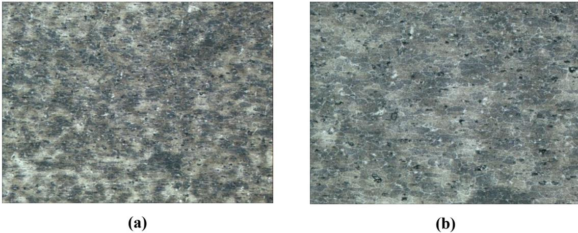
**Figure 9 (a) Magnification 100X; (b) Magnification 200X on Grain Structure of 1055 RPM Sample**
