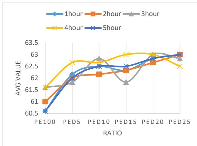
**Figure 31: Average Shore D hardness for PED after UV irradiation at 70°C for the duration of 1 to 5 hours**
