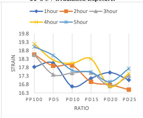
Figure 17: The average strain vs ratio for PD at 70°C UV Irradiation Exposure.
