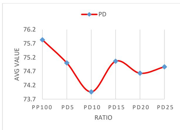
Figure 24: Shore D hardness for PD before UV irradiation
