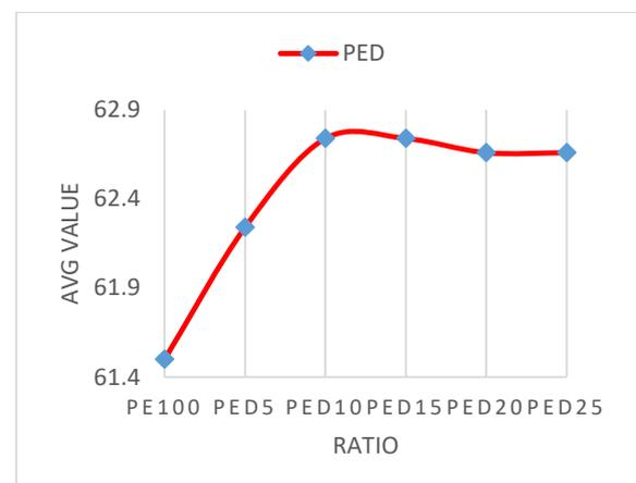
Figure 25: Shore D hardness for PED before UV irradiation
