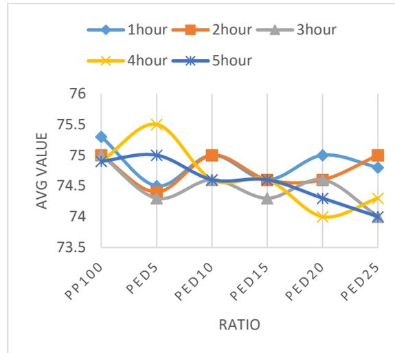
**Figure 27: Average Shore D hardness for PD after UV irradiation at 60°C for the duration of 1 to 5 hours.**
