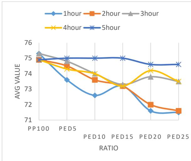
**Figure 26: Average Shore D hardness for PD after UV irradiation at 50°C for the duration of 1 to 5 hours.**
