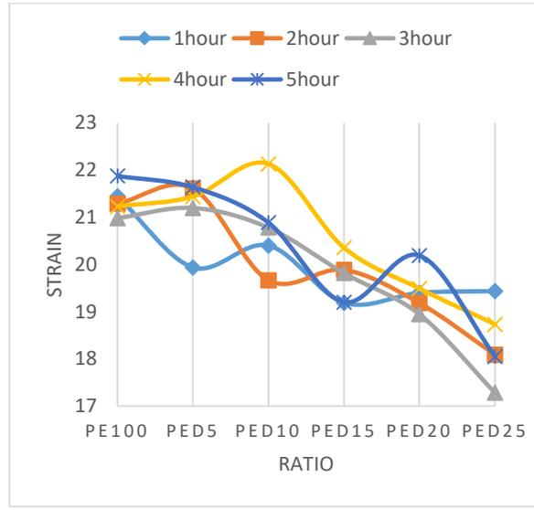
**Figure 19: The average strain vs time for PED at 50°C UV Irradiation Exposure**
