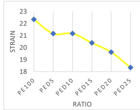
Figure 11: Strain vs ratio for PE<sub>100</sub> and PED.
