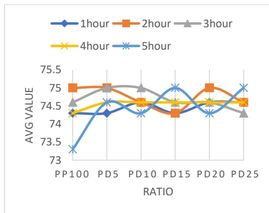
**Figure 28: Average Shore D hardness for PD after UV irradiation at 70°C for the duration of 1 to 5 hours.**
