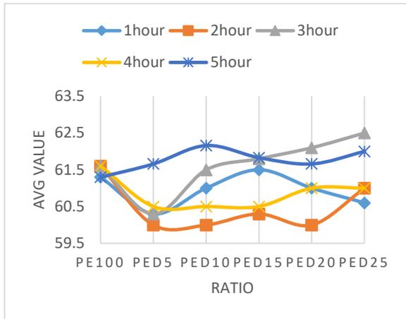
**Figure 29: Average Shore D hardness for PED after UV irradiation at 50°C for the duration of 1 to 5 hours.**
