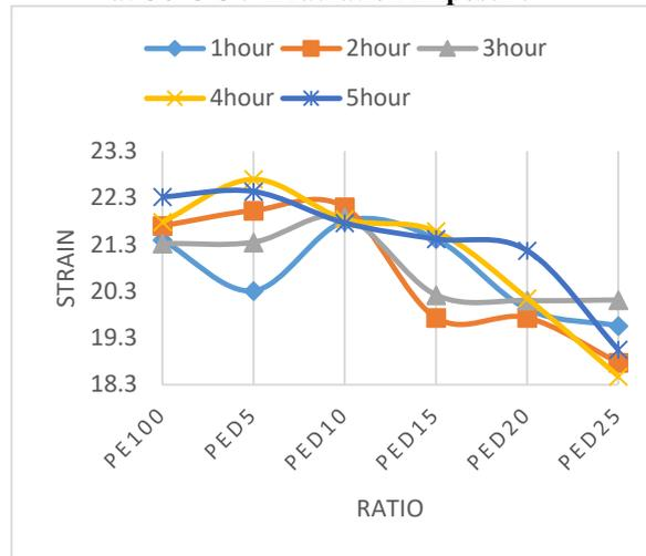
**Figure 21: The average strain vs ratio for PED at 60°C UV Irradiation Exposure**
