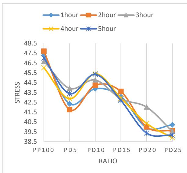
Figure 12: The average stress vs ratio for PD at 50°C UV Irradiation Exposure.
