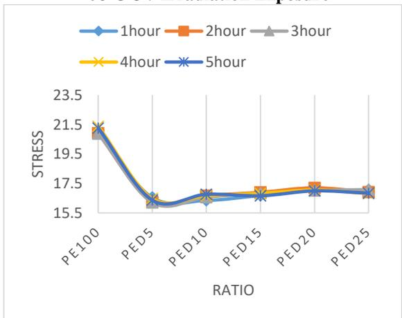
**Figure 22: The average stress vs ratio for PED at 70°C UV Irradiation Exposure**
