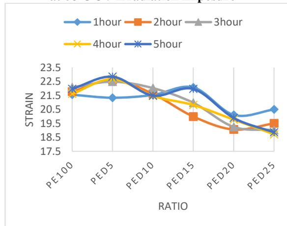
**Figure 23: The average strain vs ratio for PED at 70°C UV Irradiation Exposure**
