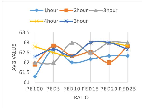
**Figure 30: Average Shore D hardness for PED after UV irradiation at 60°C for the duration of 1 to 5 hours.**
