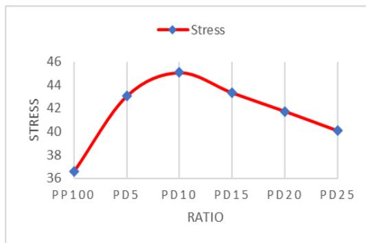
Figure 8: Stress vs ratio for  $PP_{100}$  and  $PD$ .
