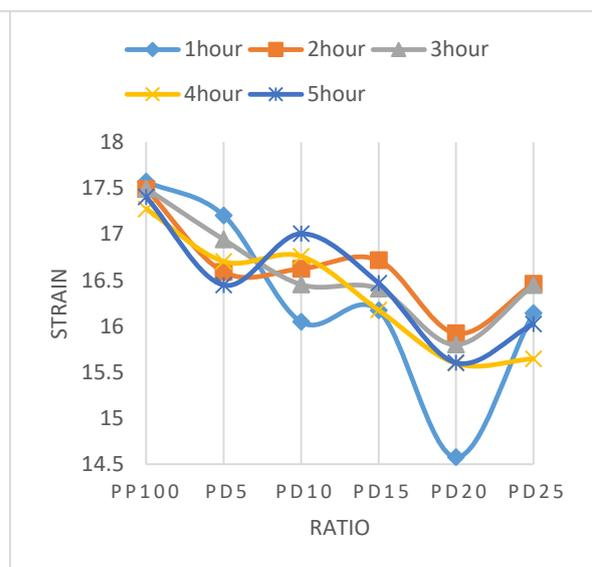
Figure 13: The average strain vs ratio for PD at 50°C UV Irradiation Exposure.
