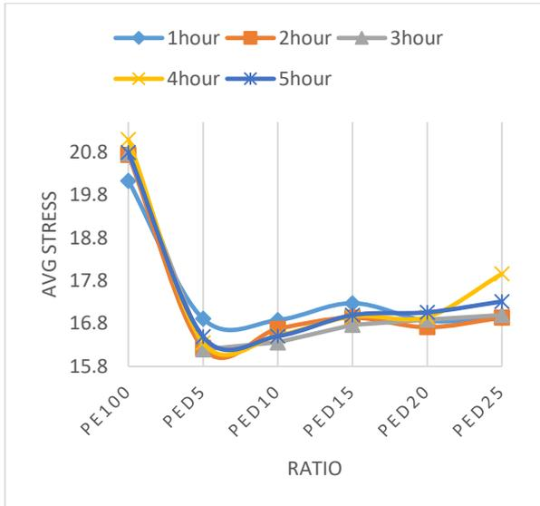
**Figure 18: The average stress vs ratio for PED at 50°C UV Irradiation Exposure**
