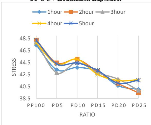
Figure 16: The average stress vs ratio for PD at 70°C UV Irradiation Exposure.
