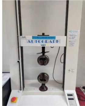
**Figure 6: Universal testing machine**
