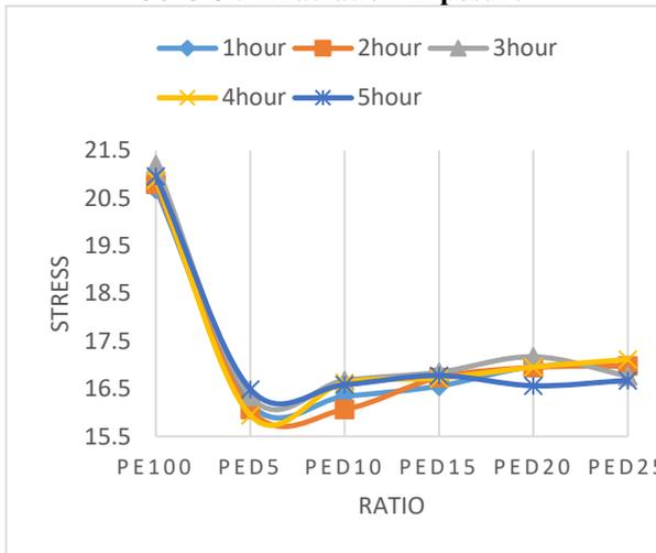
**Figure 20: The average stress vs ratio for PED at 60°C UV Irradiation Exposure**
