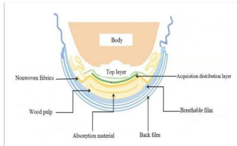
**Figure 3: Structure of a disposable diapers**
