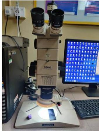
Figure 7: Olympus SZH10 Optical Microscope
