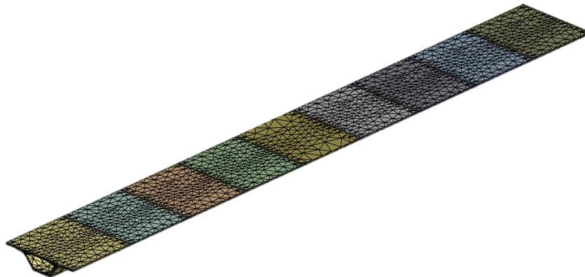
Figure 4 Finite element model of girder.
