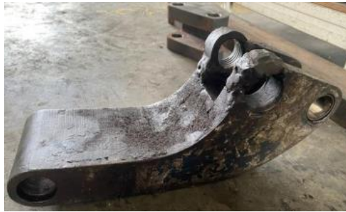
Figure 1: Broken bending arm
