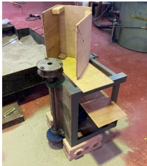
Figure 1: Centrifugal Casting completely set up
