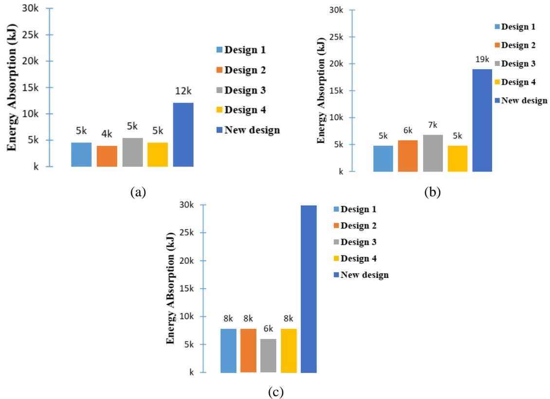
Figure 5: Energy absorption of different designs subjected to different velocities, (a) 12.5m/s, (b) 15.0 m/s, and (c) 17.5m/s
