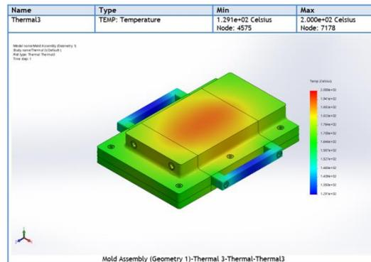
**Figure 5: Thermal analysis result for the 200°C temperature**
