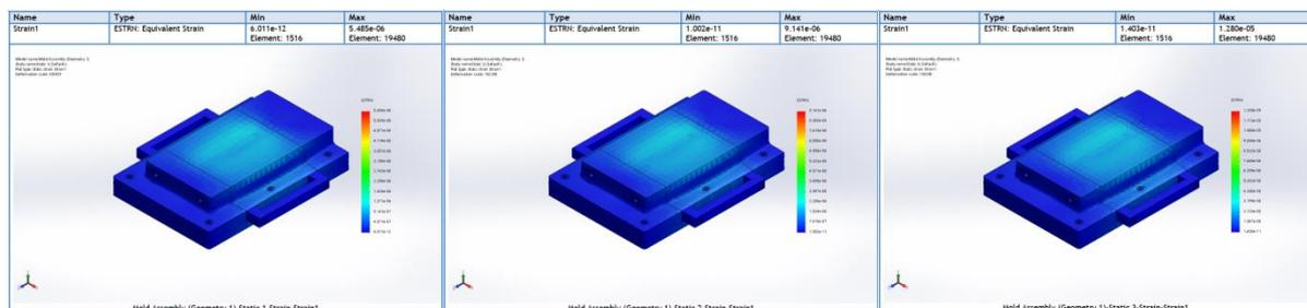
Figure 10: Pressure analysis result of the strain for (a) 3bar (b) 5 bar (c) 7 bar
