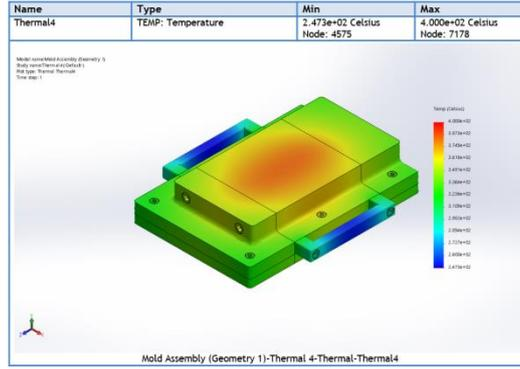
Figure 6: Thermal analysis result for the 400°C temperature
