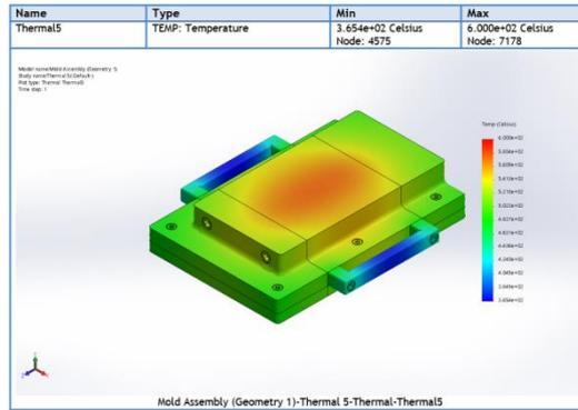
Figure 7: Thermal analysis result for the 600°C temperature
