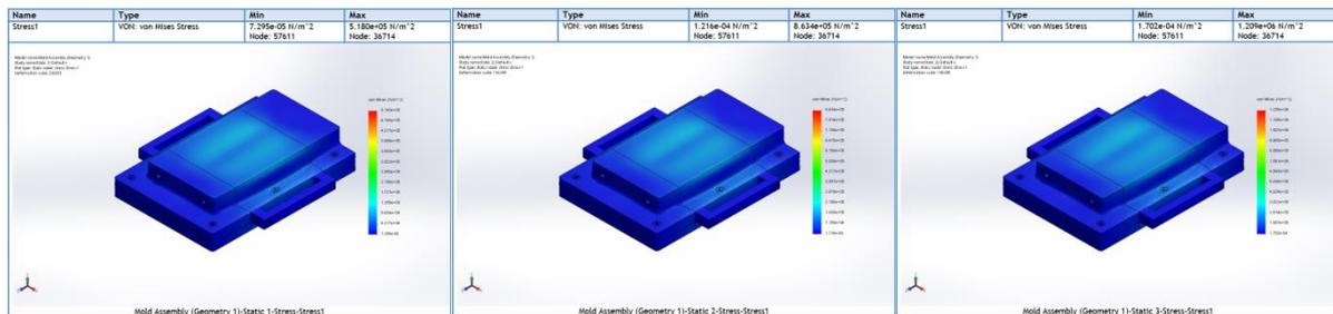
Figure 8: Pressure analysis result of the stress for (a) 3bar (b) 5 bar (c) 7 bar
