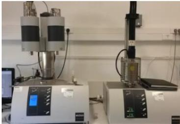
**Figure 1: TGA and DSC machine**
