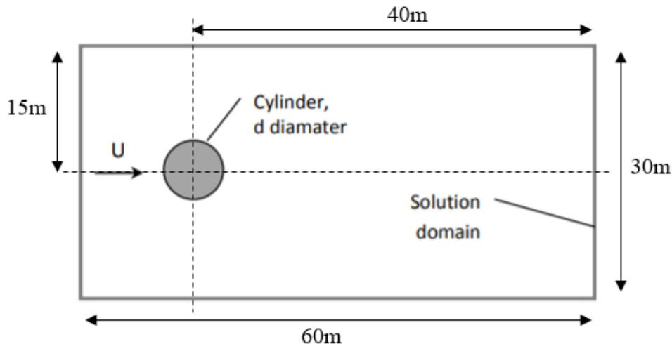
**Figure 1: Plan view of 2D model of vortex bladeless wind turbine**
