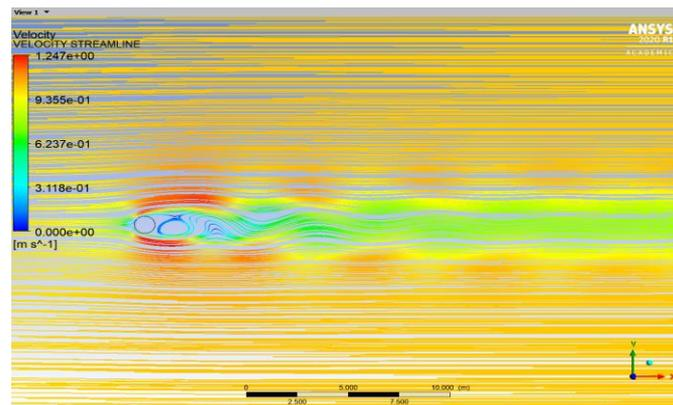
**Figure 8: Velocity streamline around the cylinder**
