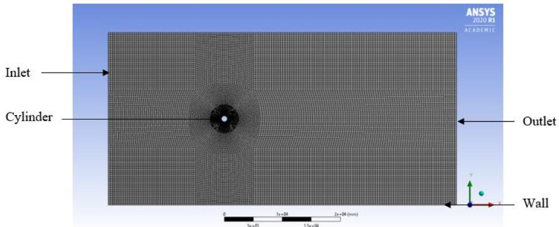
**Figure 3: Rectangular domain with smooth quadrilateral grids for the meshing**
