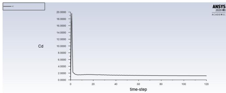
**Figure 7:  $C_d$  against flow-time graph**
