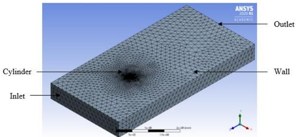
**Figure 6: Meshing of 3D model with boundary name of the solution domain**
