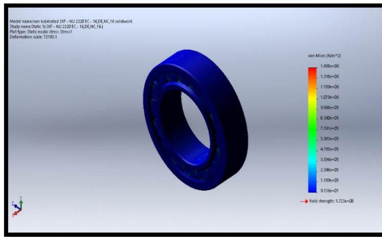
**Figure 3: Equivalent force on the cylindrical roller bearing without lubrication by SOLIDWORKS**
