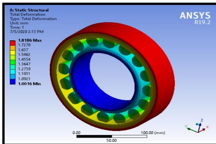
**Figure 6: Total deformation on the cylindrical roller bearing using grease lubrication**
