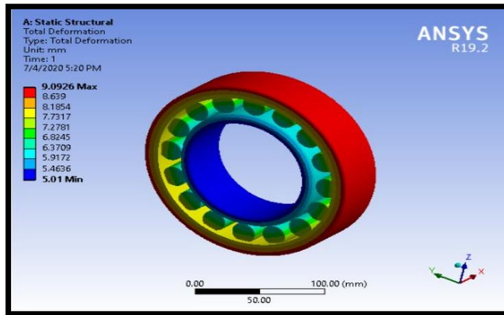
**Figure 5: The total deformation on the cylindrical roller bearing without lubrication by ANSYS**
