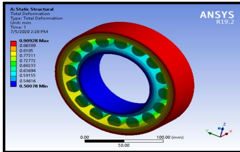
**Figure 7: Total deformation on the cylindrical roller bearing using oil lubrication**
