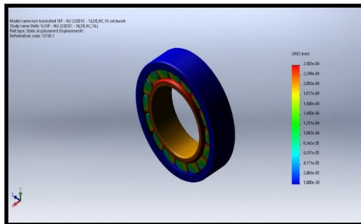
**Figure 4: Total deformation on the cylindrical roller bearing without lubrication by SOLIDWORKS**
