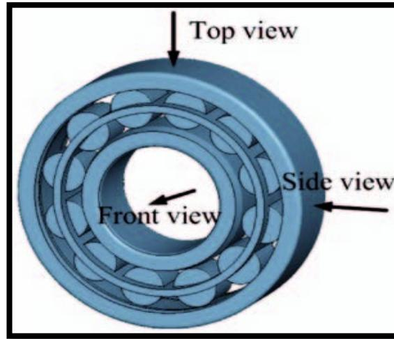
**Figure 1: Schematic of a cylindrical roller bearing [5]**
