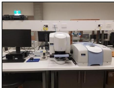
**Figure 4: Perkin Elmer 100 Series FTIR spectroscopy**
