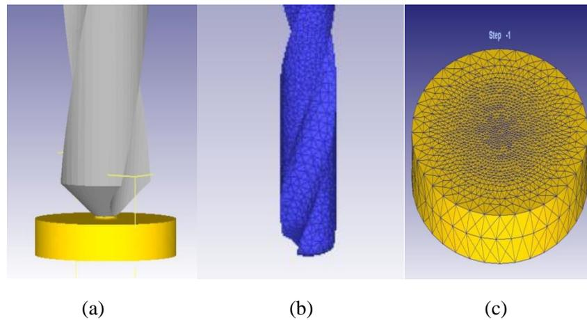
**Figure 1: (a-c); (a) Geometric model, (b) Mesh of drill bit, (c) Mesh of workpiece**
