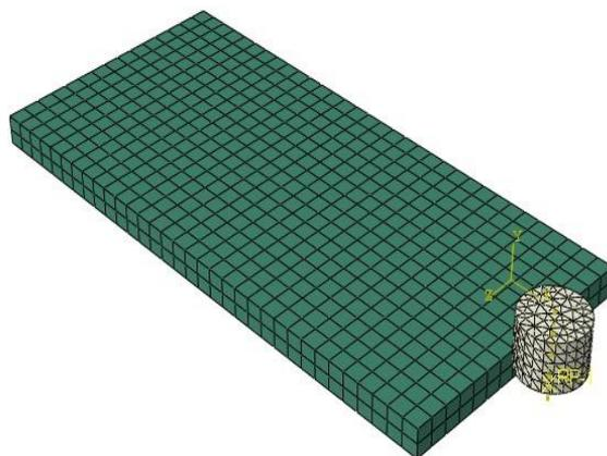
**Figure 2: Example of C3B8T Mesh on Workpiece**
