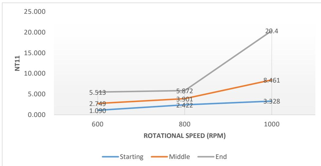
Figure 4: NT11 result on Mg\_Alloy Plate
