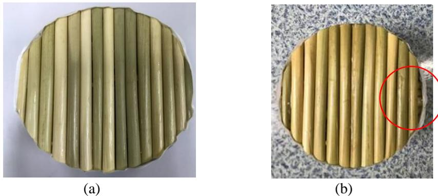
**Figure 2: Samples made up of *Lepironia articulata* with diameter ranging from 4 to 7 mm for (a) Horizontal arrangement and (b) Crossed arrangement where succession of alternate layers is clearly visible inside the red circle.**
